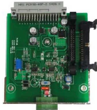
Analog Output (4–20mA, 0–10V)
