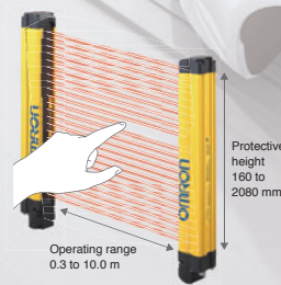
F3SG-4RE □□□□-14 Detection capability: Dia. 14 mm
