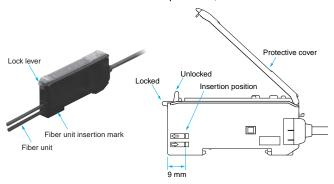
Note: Do not pull on the fiber unit, apply pressure on it, or otherwise subject it to excessive force when it is attached to the Amplifier Unit.
