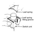
**Note:** Be sure to fit the leaf spring exactly into the groove, and do not allow it to slip out of the groove.
