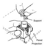
**Note:** Completely remove any burrs on the panel cutout surface; otherwise, the flange and switch unit will not attach solidly.
